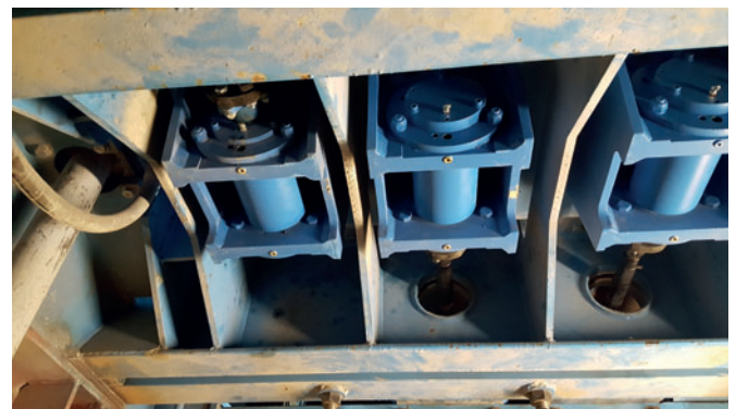
Axis Vibrosystem modification without replacing the table in Tüßling, Germany
