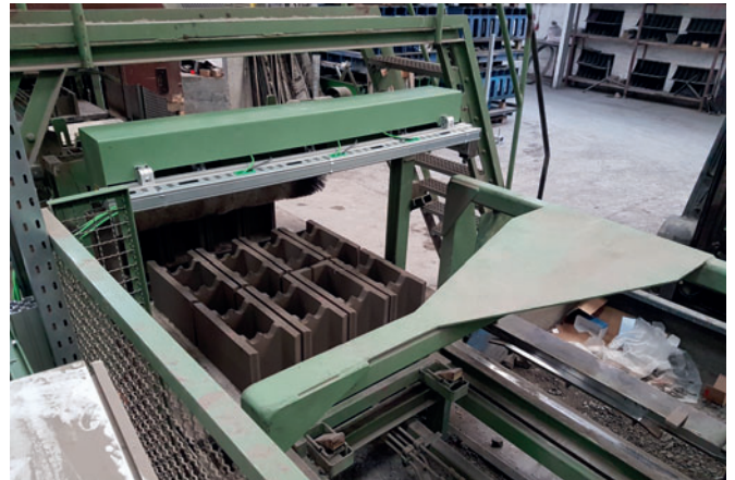
Block height measurement system in East Germany
