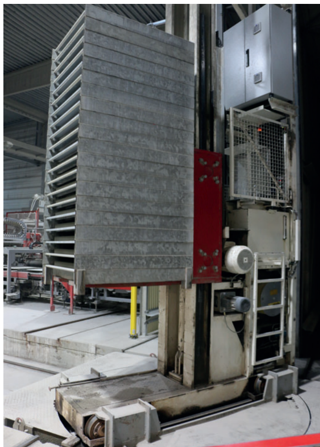
Control unit modification of a mobile elevator for a slab press in Fensterbach, Germany
