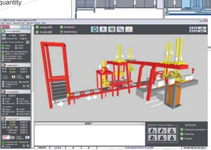
The visual system is connected to the PLC by the fast Profinet (Ethernet).
