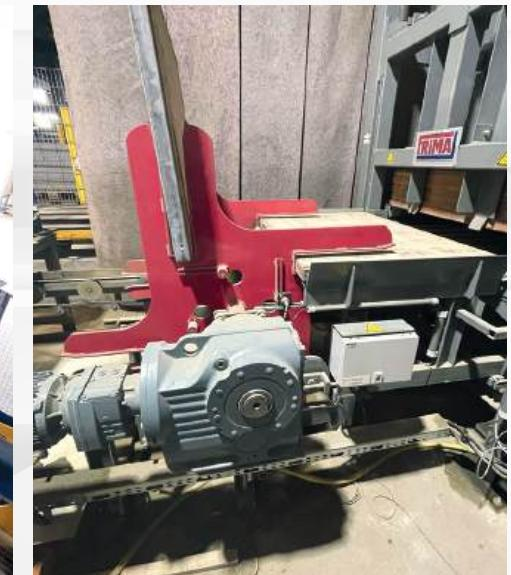
Systems for returning the empty boards from the dry to the wet side with board buffer systems. This means that the wet and dry sides can produce independently of each other.
