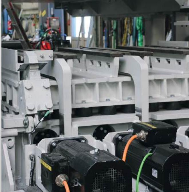
With the **FRIMA Axis vibration system** as a single table with **4 drives** or as a double table with **8 drives**, we offer our customers one of the most innovative solutions for compacting earth-moist concrete.
