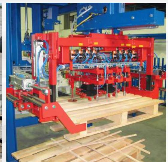
In the stone cube conveyor area, shipping pallets often have to be fed in or wooden strips inserted between the stone layers for protection of the surface.
