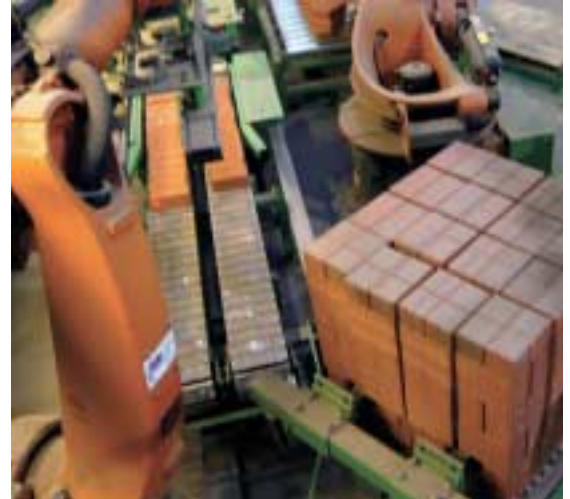
Fig 4 Robot 1 takes the blocks and forms a double row.
