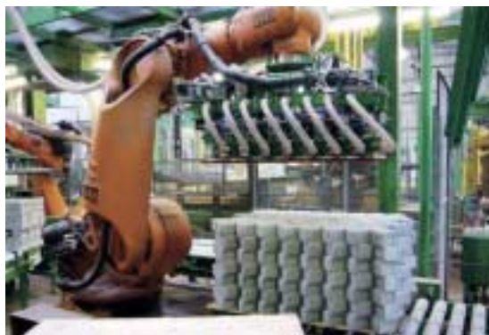
Fig. 2 Block package in herringbone pattern.
