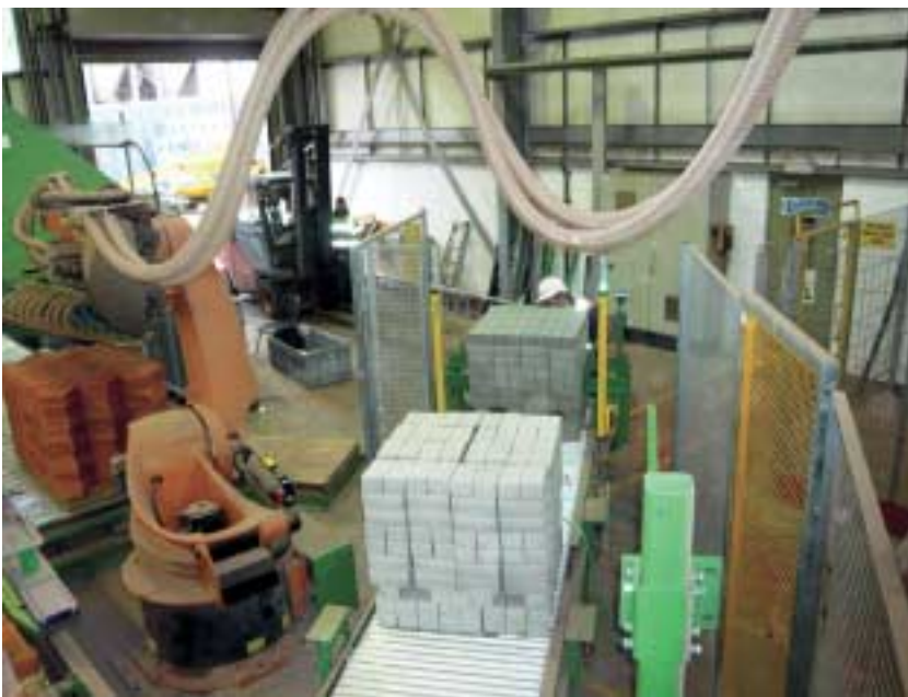
Fig. 1 Loading of the roller conveyor with block packages. These packages will be reformatted into herringbone pattern.
